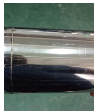
Gas-Tight Cylindrical Structure Welding
