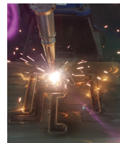
Intake and Exhaust System Welding
