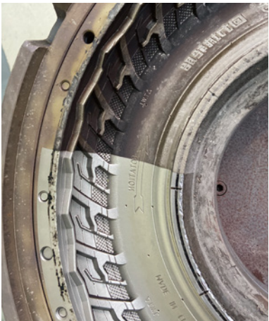
Mold Oil & Residue Cleaning
