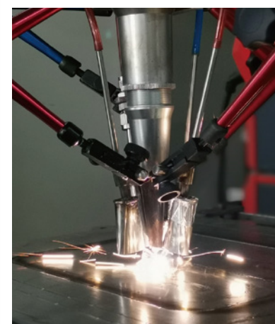
Battery Structure Welding
